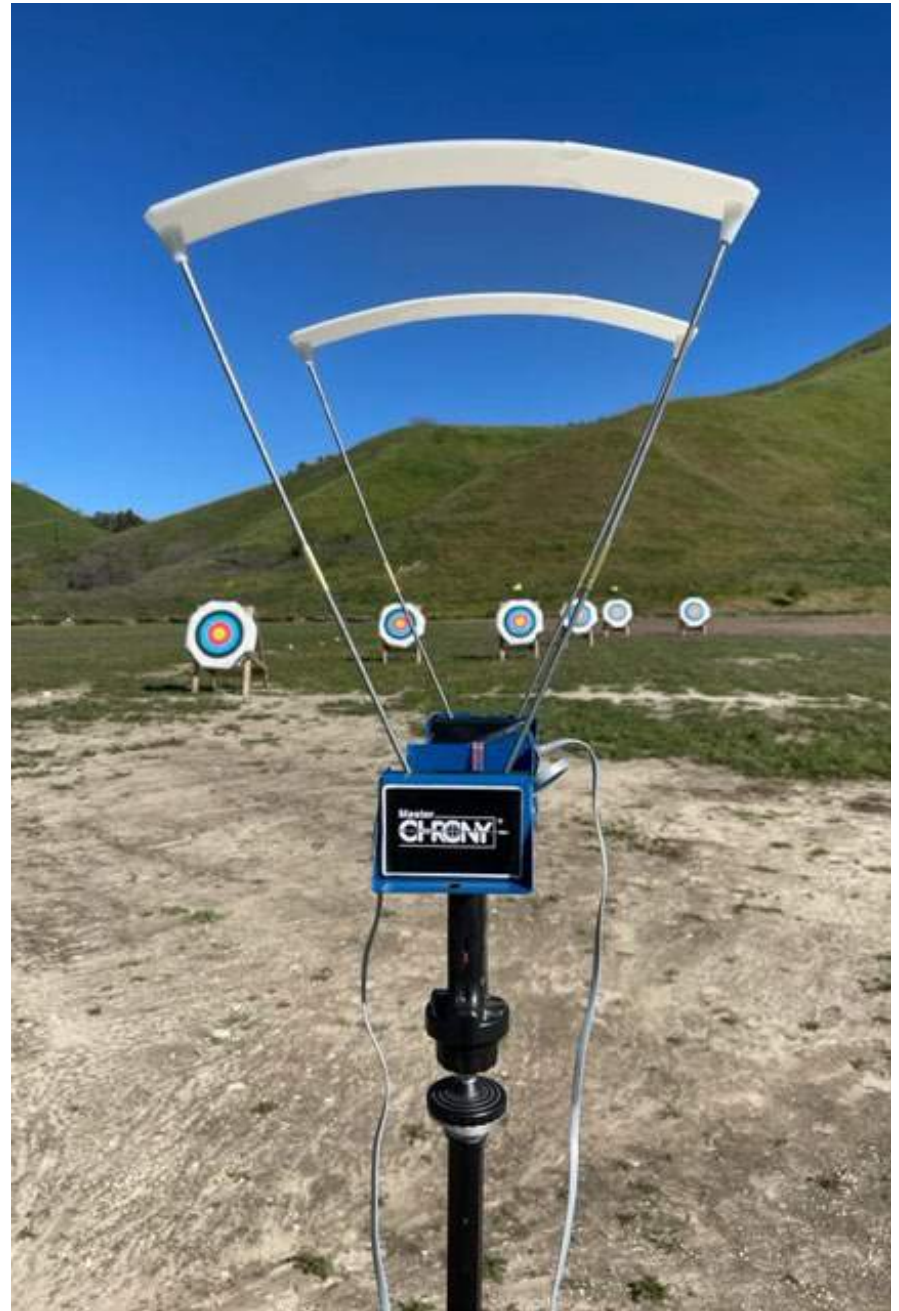
What is this? Trying to get radio waves at the range? Nope, Ken is measuring arrow speed using his chronograph.
